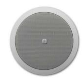
The CM20T two-way built-in loudspeaker can be used as a 16 ohms or 100 volt loudspeaker. In 16 ohms use, you can connect up to 4 loudspeakers in parallel on each channel of a standard 4 ohms amplifier. For 100 volt use, the CM20T is equipped with a high-quality 20 watts 100 volt transformer with several power tappings (20 - 10 - 5 - 2.5 watts). Therefore it can be used in projects with high ceilings or places with background noise where a little more power is needed.
